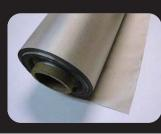
Spec Surface Resistivity: 0.03 Ohm/sq characteristics high conductivity. Superior tarnish and corrosion resistance due to Nickel content. Nickel may produce skin allergies active component Copper and Nickel method coated textile material nylon
