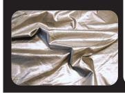
Spec Surface resistivity: < 0.25 Ohm/sq characteristics high conductivity active component
